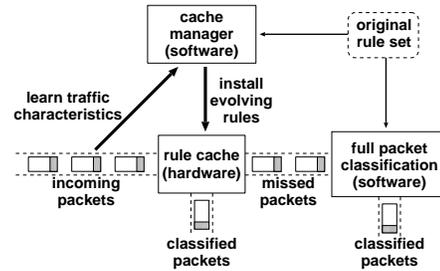
**Figure 2: Framework of the smart rule cache.**
