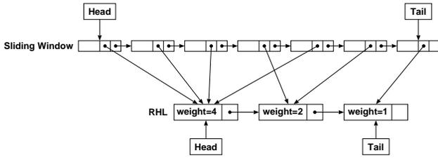
Figure 4: Data structures of smart rule cache.
