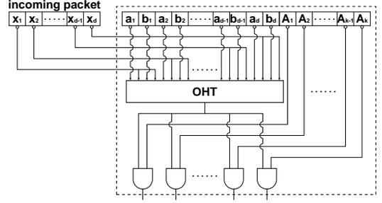
Figure 8: Hardware design of a cache entry.
