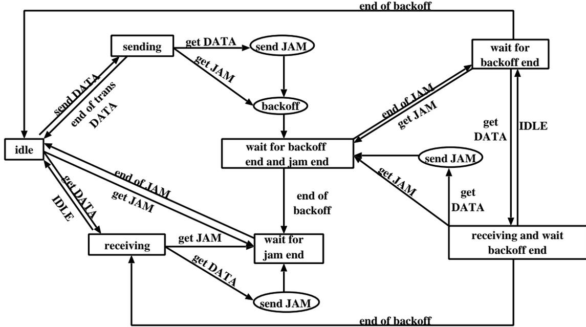
Figure 3: State diagram of distributed CSMA/CD simulation
