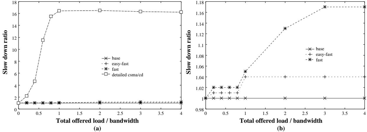
Figure 13: The ratio of CPU time consumed for 10 seconds simulations of 10 Mbps Ethernet link with packet size = 512 bytes and buffer size = 8 packets ((b) is the zoomed version of the three curves in the lower portion of (a)).
