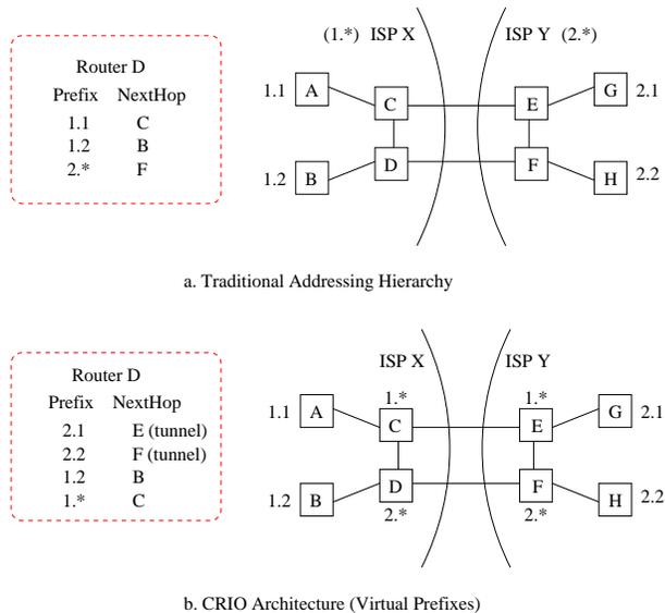
Fig. 1. An example of traditional hierarchy and CRIO using a simple 2-level hierarchical address
