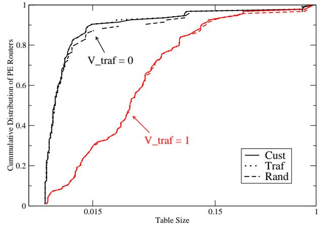
Fig. 8. Comparison between different virtual prefix placement schemes
